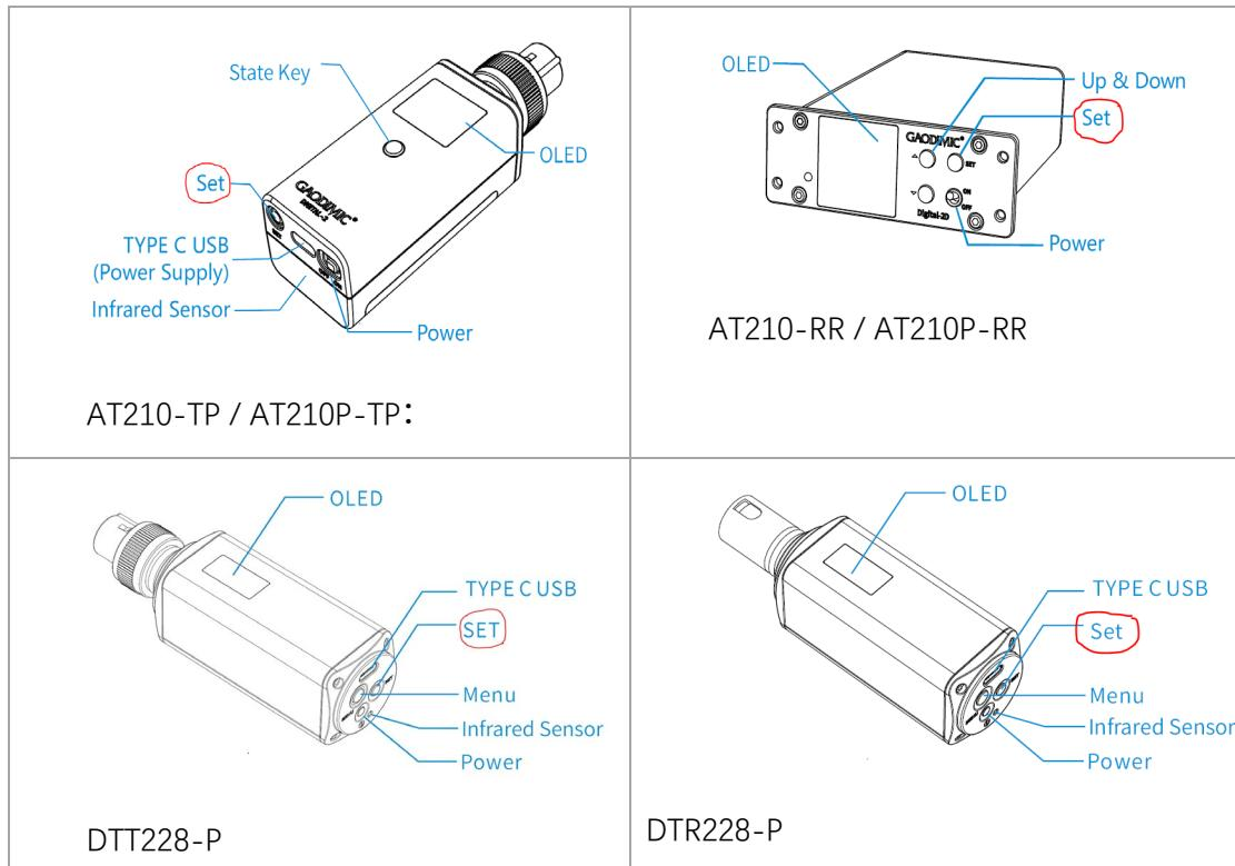
Scenarios 2: Long press other keys while turning on the device. The following products are suitable for this method:
